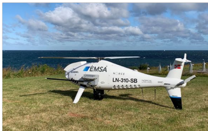
EMSA, larger drone with mini sniffer
