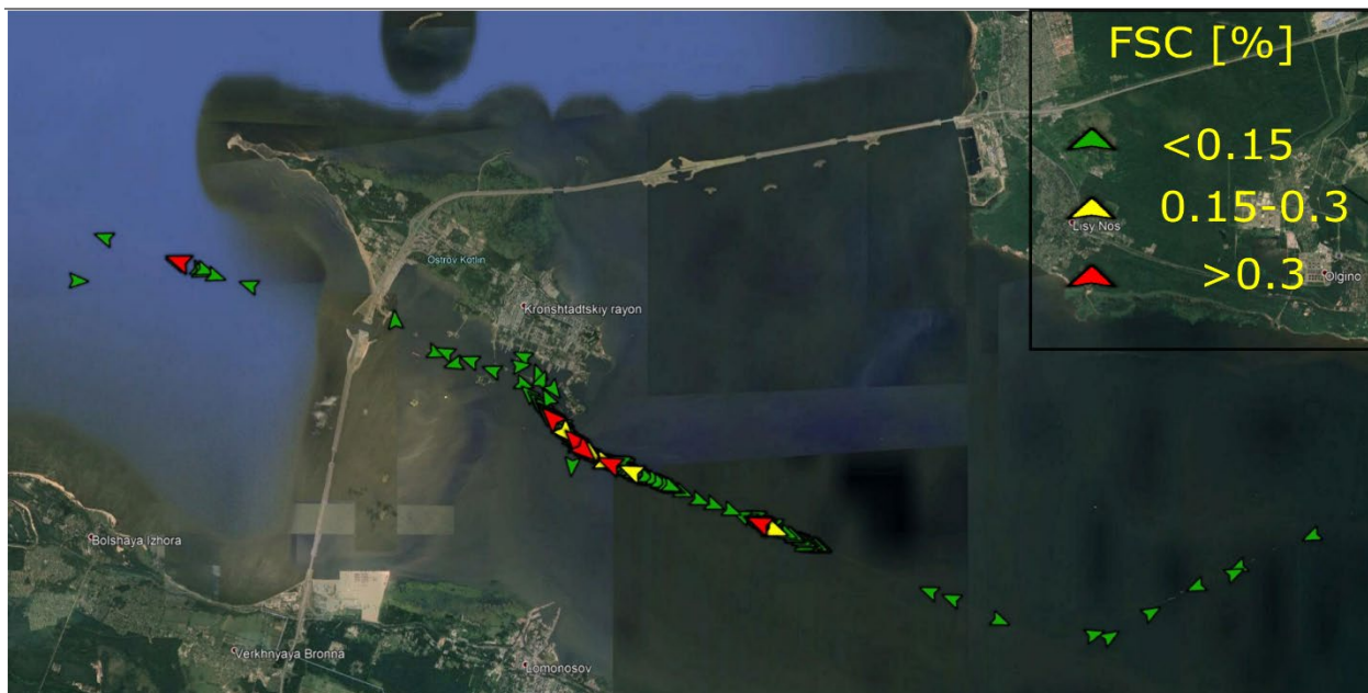
Figure 9. Shipborne FSC measurements of individual ships in Neva bay, St Petersburg in the EnviSum project. The FSC limit for detected non-compliance is here 0.15%, taking into account the measurements error.
