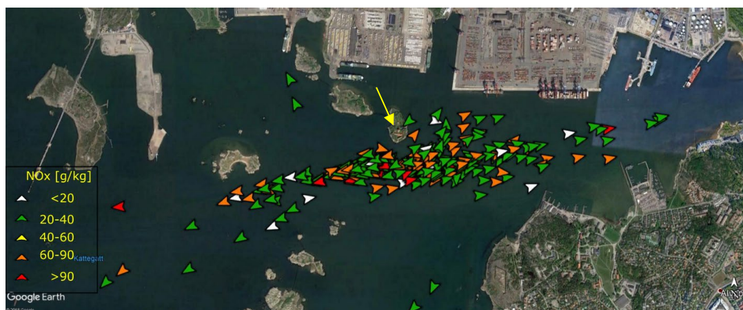
Figure 13. The mass specific emission of NO x (g/kg fuel ) in individual ships upwind of the Älvsborg site (yellow arrow), close to the Göteborg ship channel.
