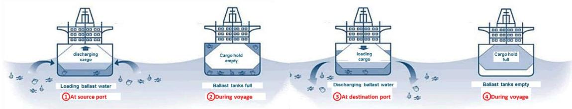
Figure 8 Ballast water cycle through a voyage.
